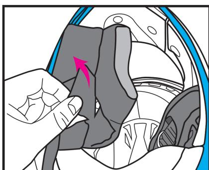
4. Put the chin strap into the holes of cheek pad liner.
