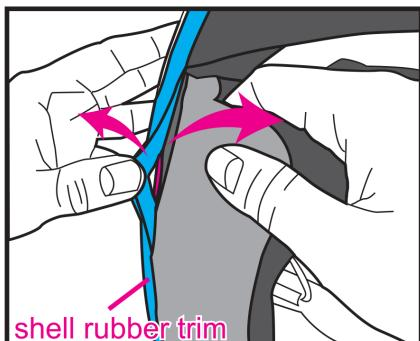
1. Grasp the shell rubber trim, then remove the PE board of cheek pad liner from the shell.
