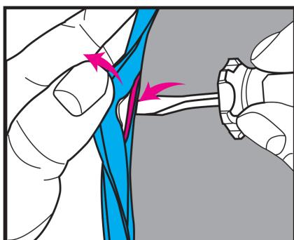
3. Adjust the position of cheek pad liner, grasp the shell rubber trim, then tool in order to fix all the PE board into the interior shell rubber trim.
