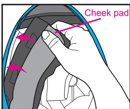
2. Put the PE board of new cheek pad liner and insert into the shell & cheek pad EPS in between.
